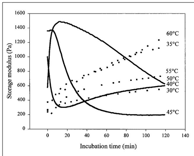
**Fig. 4—Gel elasticity ( $G'$ ) of paddlefish surimi sol (40 mg/mL protein, 2.5% NaCl, pH 6.5) incubated at selected temperatures for 2 h. (Solid lines show the  $G'$  with declining trend from the initial peak; dotted lines show the  $G'$  with increasing trend).**
