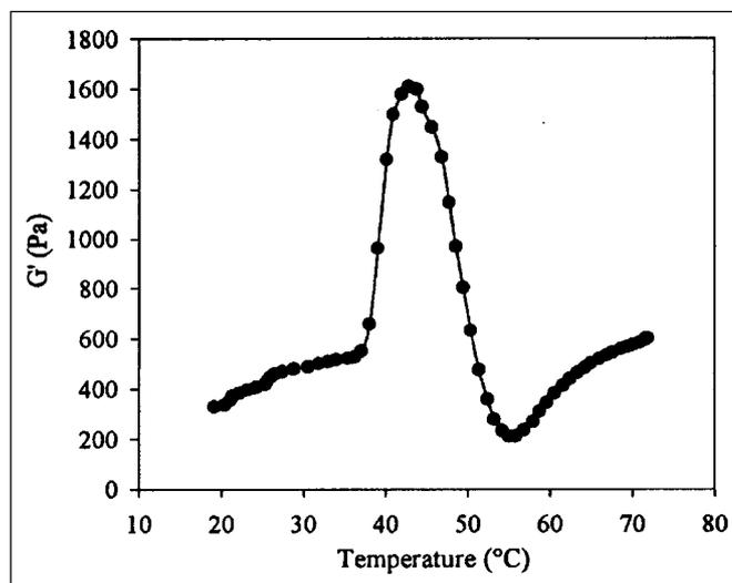
**Fig. 3**—Typical rheogram of paddlefish surimi sol (40 mg/mL protein, 2.5% NaCl, pH 6.5) heated from  $20\text{ }^{\circ}\text{C}$  to  $73\text{ }^{\circ}\text{C}$  at  $1\text{ }^{\circ}\text{C}/\text{min}$ .
