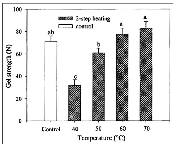
**Fig. 2**—Gel strength of paddlefish surimi (180 mg/mL protein, 2.5% NaCl, pH 6.5) pre-incubated at selected temperature for 30 min followed by final cooking at  $90\text{ }^{\circ}\text{C}$  for 30 min (Mean  $\pm$  SE). The control was cooked in a  $90\text{ }^{\circ}\text{C}$  water bath directly. The bars sharing the same letter a, b, or c were not significantly different.
